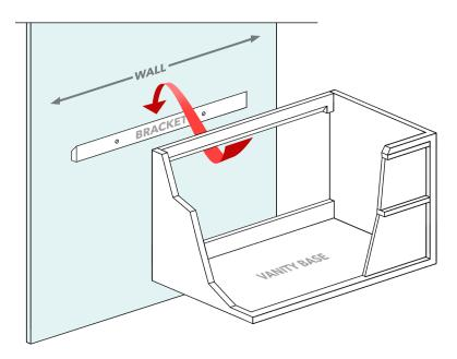
5. While two people hold the vanity base (D) in place, the third person marks screw placement in the top and bottom rails in the back of the vanity, making sure they are in line with the screws in the hanger and aligned with the studs. Then drill guide holes and secure vanity to the wall with lag screws (F) and washers (G).
