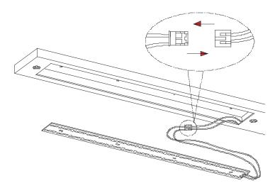
3. Unplug the connector and replace the LED strip.
