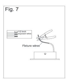
7. Use a pair of wire stripper to remove about 1/2" inch of insulation from each wire.
