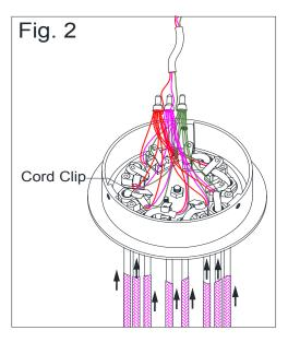
2. Determine the hanging length for light, pull the hanging cords out through the cord clips to desired length.
