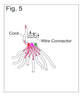
5. Remove the wire connectors using the plier.
