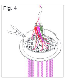
4. Cut off the pulled out cords with the wire cutter provided.
