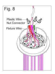
8. Reconnect the wire ends and secure with the plastic nut connectors.
