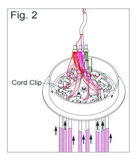
Determine the hanging length for light,pull the hanging cords out through the cord clips to desired length.
