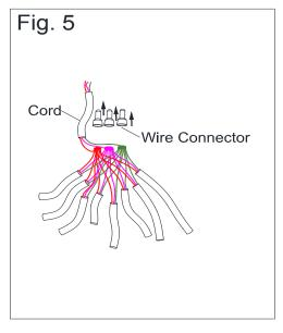
5. Remove the wire connectors using the plier.
