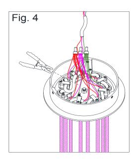
4. Cut off the pulled out cords with the wire cutter provided.
