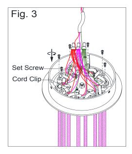
3. Replace the set screws and tighten to lock the hanging cord in place.
