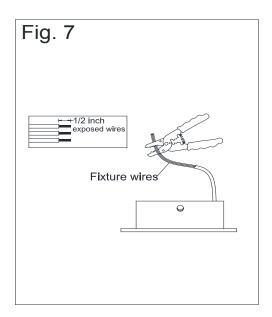
7. Use a pair of wire stripper to remove about 1/2" inch of insulation from each wire.
