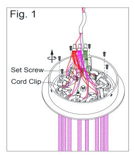
1. Loosen set screws on the top of the cord clips.
