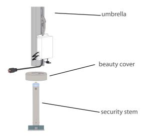
Step 4 lock umbrella down by pushing the cam lock handle in the down position and reinsert the pin. Mount beauty cover over control box.
