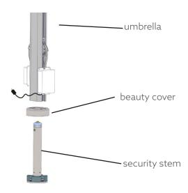
Step 4 lock umbrella down by pushing the cam lock handles in the down position and lock with pins. Mount beauty covers over control boxes.
